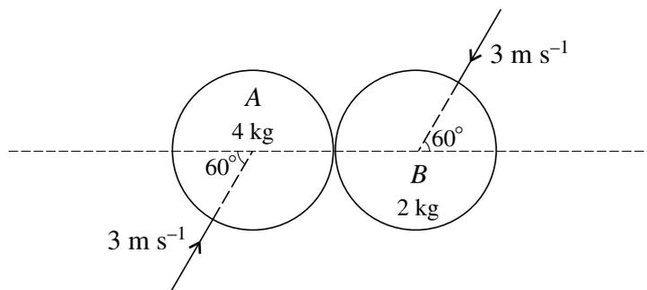
Two uniform smooth spheres  $A$  and  $B$ , of equal radius, have masses  $4 \text{ kg}$  and  $2 \text{ kg}$  respectively. They are moving on a horizontal surface when they collide. Immediately before the collision both spheres have speed  $3 \text{ m s}^{-1}$ . The spheres are moving in opposite directions, each at  $60^\circ$  to the line of centres (see diagram). After the collision  $A$  moves in a direction perpendicular to the line of centres.
