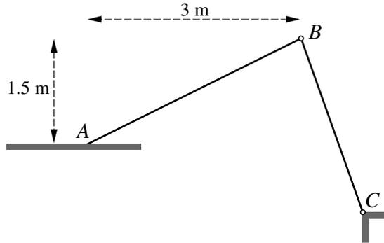
Two uniform rods,  $AB$  and  $BC$ , are freely jointed to each other at  $B$ , and  $C$  is freely jointed to a fixed point. The rods are in equilibrium in a vertical plane with  $A$  resting on a rough horizontal surface. This surface is  $1.5 \text{ m}$  below the level of  $B$  and the horizontal distance between  $A$  and  $B$  is  $3 \text{ m}$  (see diagram). The weight of  $AB$  is  $80 \text{ N}$  and the frictional force acting on  $AB$  at  $A$  is  $14 \text{ N}$ .
